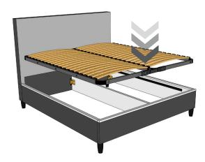
**8.** Lower the slatted frame into the bedframe making sure you move the slatted frame so that a 20mm gap is made at the head and foot end (frame is centred). Then place the 2x55mm screws (with 1x washer on each) and fix in place either side of the frame.
